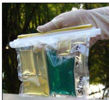
Left: Positive (blue/blue green) and negative (yellow/yellow brown) compartments indicate E. coli Right: CBT Kit includes complete supplies for 10 tests (Credit: Aquagenx)
