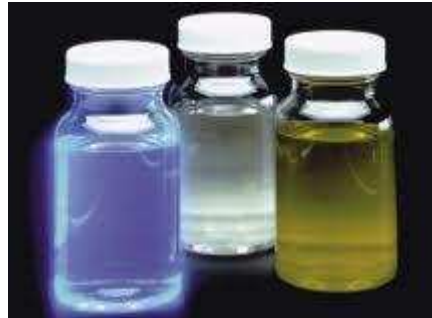
Left: Colilert package, Right: Presence-absence test bottles with positive results (Credit: IDEXX)
