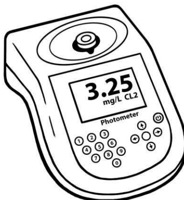
Photometer used to measure chemicals in water
