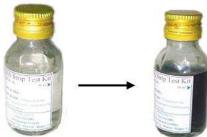
ENPHO presence-absence test bottles showing negative (clear) and positive (black) results (Credit: ENPHO)
