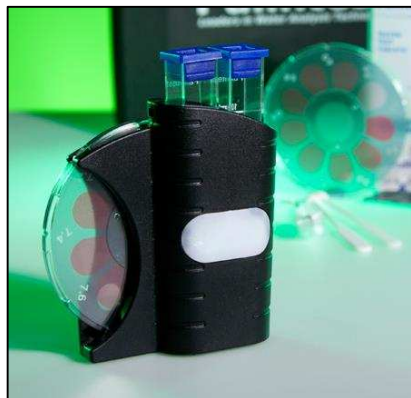
Left: Contour Comparator with test tubes and colour disc, Right: Colour disc (Credit: Palintest)
