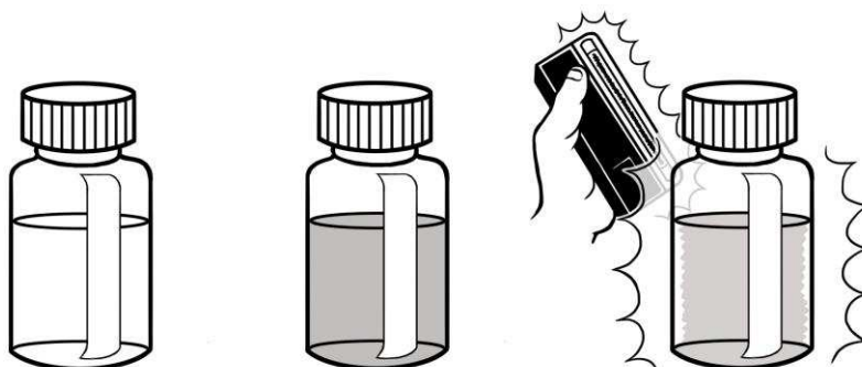
Clear water indicates a negative result for total coliforms, coloured water indicates total coliforms are present, fluorescent water indicates E. coli is present (seen using a UV lamp)
