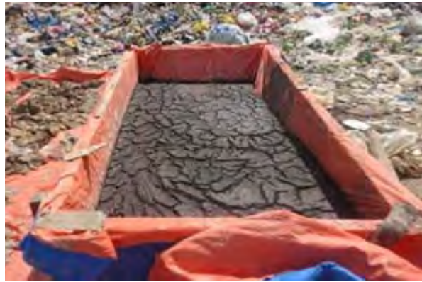
Figure 23 Dried sludge/Photo courtesy of HRC
