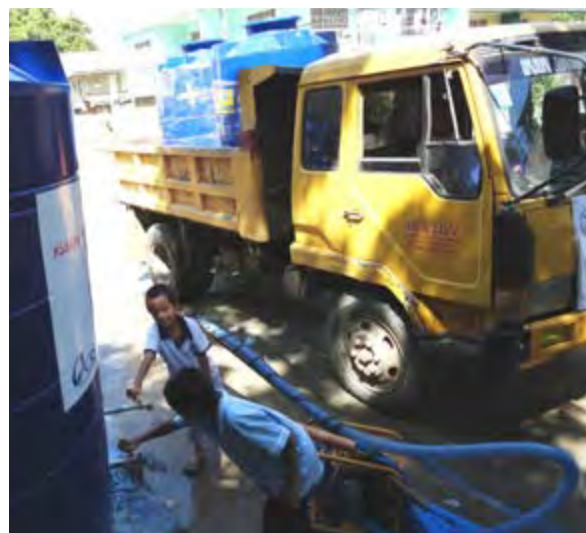
Figure 8 Water trucking using polytanks on the back of a regular truck
